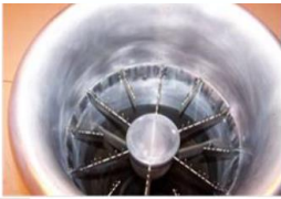
Typical intake measurement rake system • Intrusive • Low spatial fidelity
